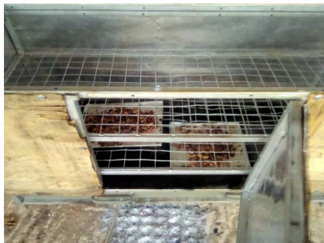
Figure 4. Cocoa beans during the drying experiment using the developed dryer
