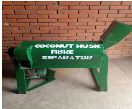
Plate 1. The Complete Coconut Husk Separator
