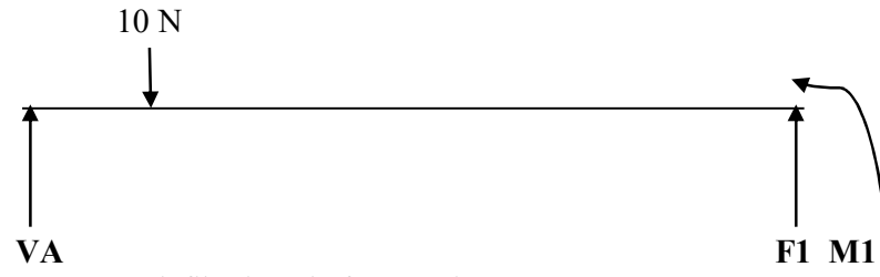
Fig. 8. Forces on defibering shaft at section 0.1 \leq X \leq 0.29
